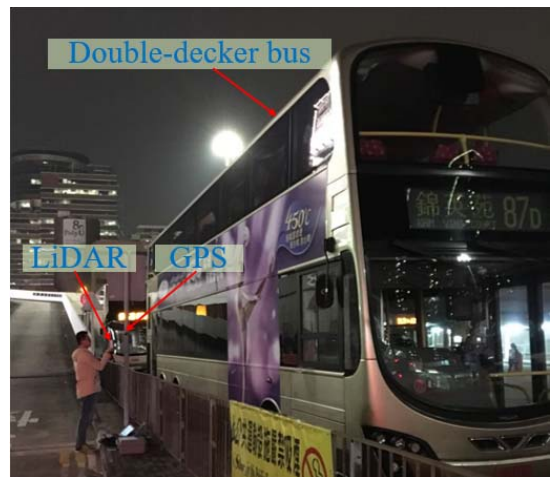
Fig. 4. Environment that the data were collected in a bus stop. Satellites can be blocked by the double-decker.
